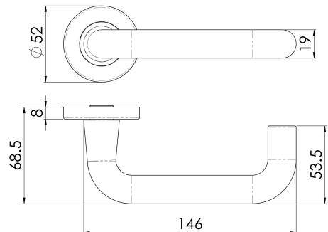
A sturdy 19mm Dia. round bar safety lever on a concealed fix press on round sprung rose. The handle returns back to the door offering reduced risk of catching clothes or injury. DDA Compliant.
