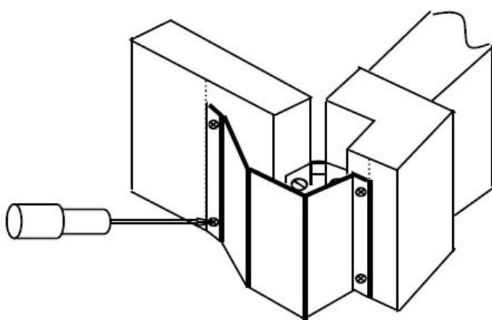
6. Repeat this procedure to attach the Finger Keeper Commercial to the door itself.
