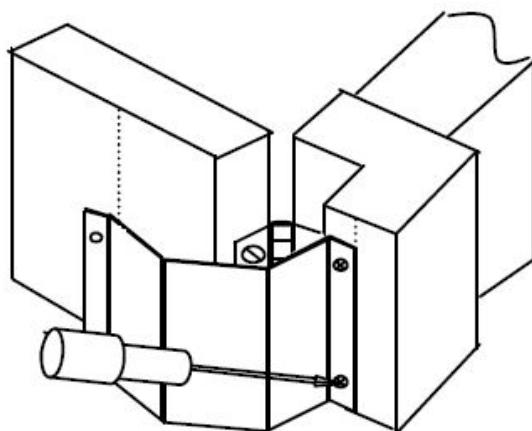
5. Line up the edge of the Finger Keeper Commercial parallel to the guideline/pencil line on the frame. Press firmly to hold in position before finally securing with Othe screws (provided). (For metal doors and kick-plates pre-drill with 2.5mm drill bit).
