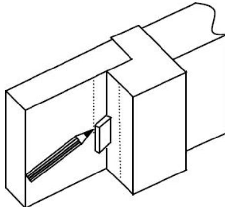
2. Simply repeat the procedure on the door to produce a second guideline.
