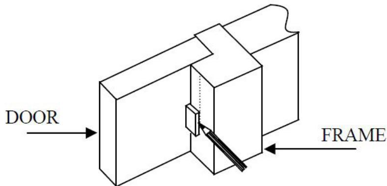
1. With the door in the closed position, use a pencil/pen to draw a guideline on the door frame using the 20mm plastic measuring block (provided).
