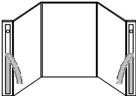
4. Remove one layer only of the double sided tape from each side of the Finger Keeper Commercial.
